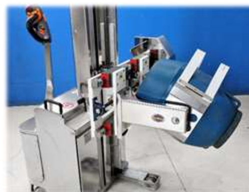
Clamps with Aisi304 stainless steel gripping equipment
