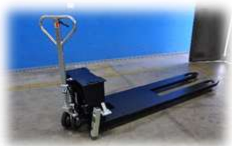
Cradle forks for reels handling.
